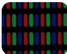
Flexible CF Array on Pylux™ MF
