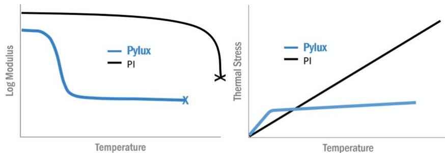
Figure 1. (a) Log-linear example plot of Young's modulus vs. temperature for Pylux™-MF and general polyimides, with thermal degradation temperatures represented by 'X's. (b) Total thermal stress in thin-films deposited atop each substrate as a function of temperature.
